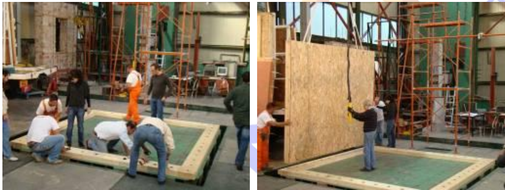
Figure. 4: Wood base to fix model on the seismic simulator.
