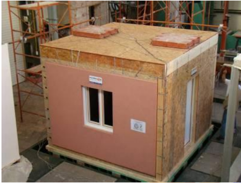
Figure. 1: Experimental layout of the model on the seismic simulator.
