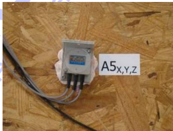
Figure. 17: Tri-axial accelerometer at position A5XYZ.
